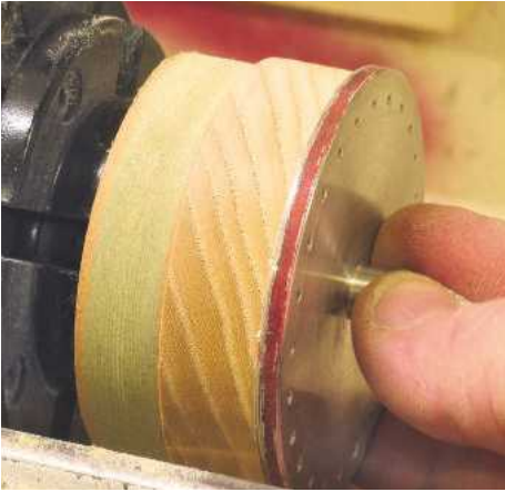
▲ Pic.10 Offering up the drilling jig to the top will give you an idea of the diameter required. Going to about 75mm, which is just below the diameter of the jig, will work better with some smaller earrings
